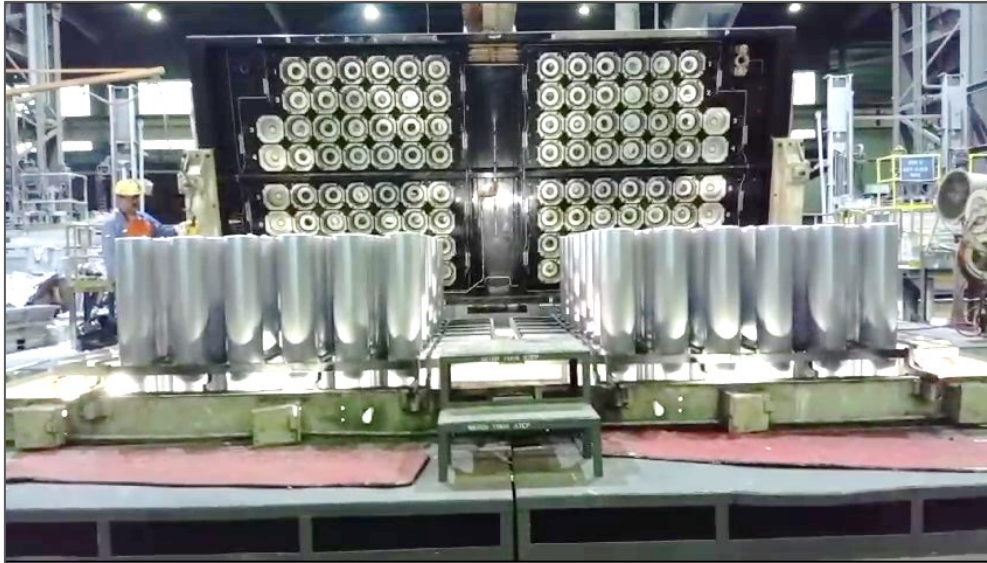
Figure 1. Air-slip casting table with mould and billets.
